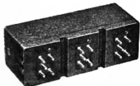
COIL UNITS (Note internal screening).
